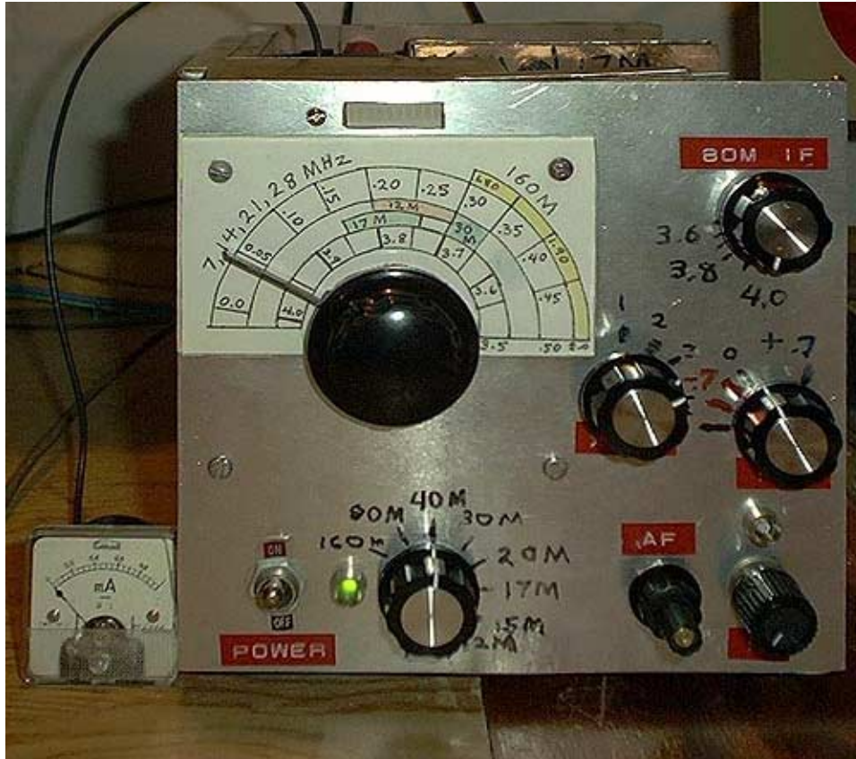
Homebuilt all-band dual conversion HF ham receiver
