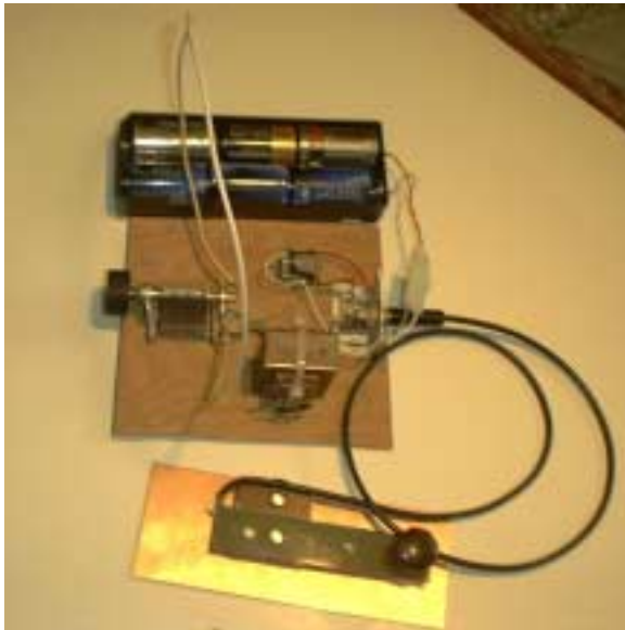
10 meter sparkgap transmitter.
