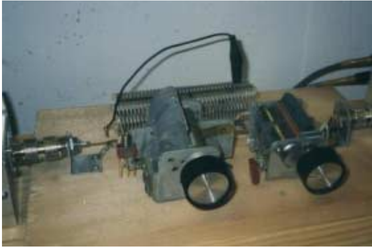
A Simple "T" Match Antenna Coupler
