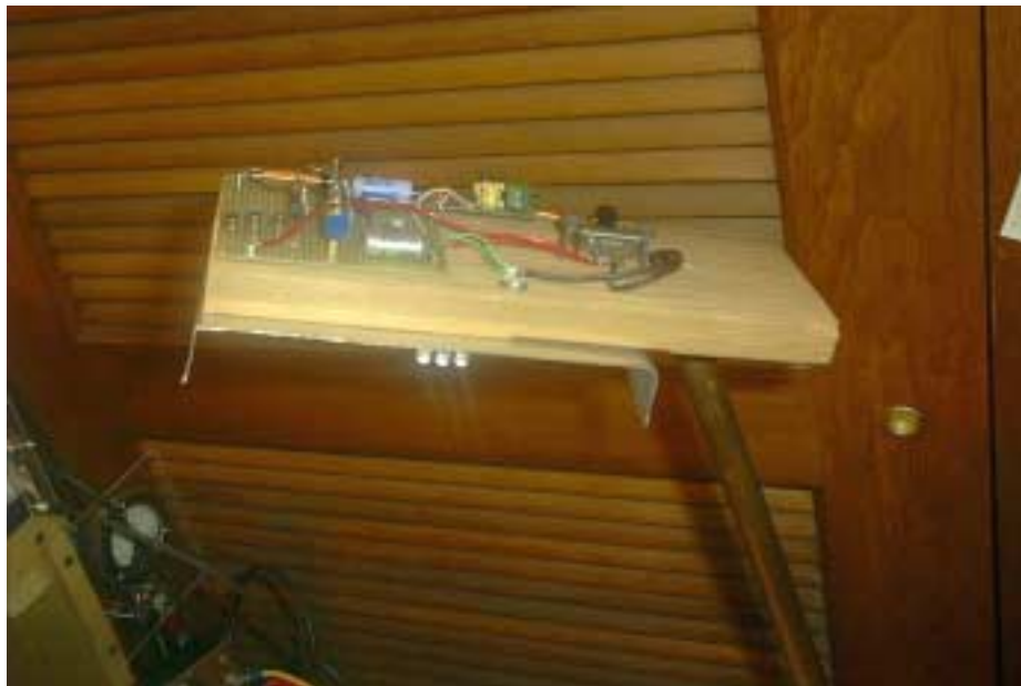
A homebrew LED and fluorescent station lamp
