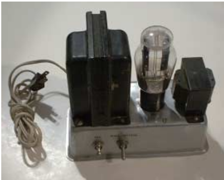
A power supply made from parts salvaged from an ancient radio.
