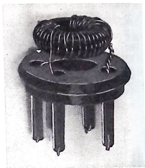
Fig. 4-6. Toroid-core transformer mounted on five-prong plug (40-meter coil).
