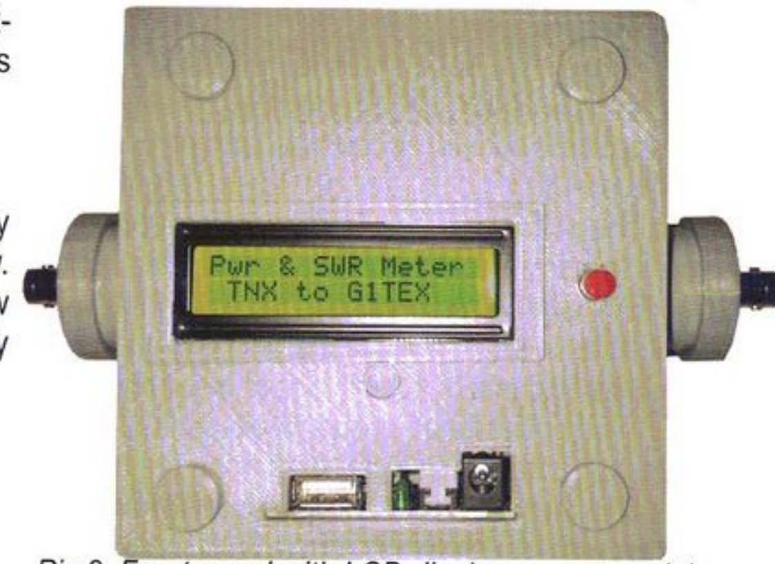
Pix 2. Front panel with LCD display, power module and 'CW' button.
