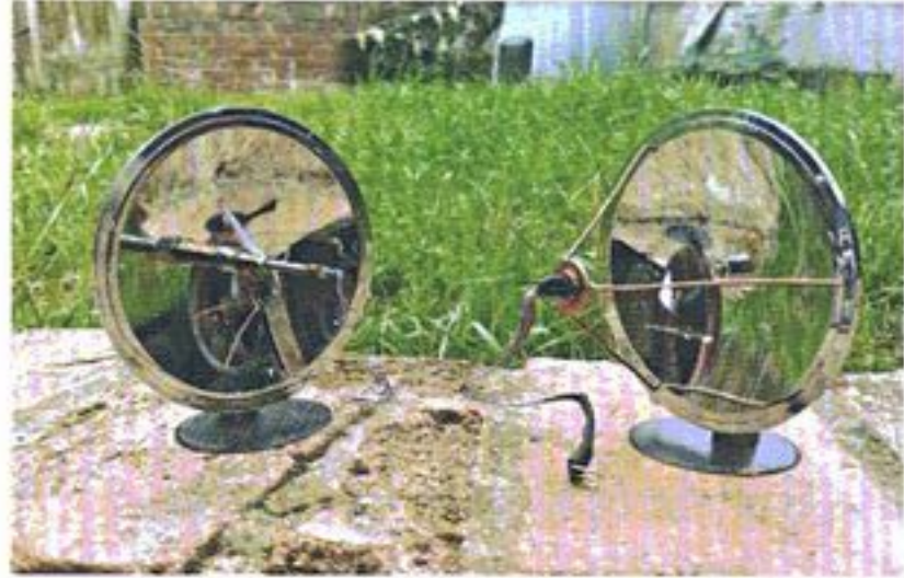
Fig. 2. Transmitter antenna (left), Receiver antenna (right)
