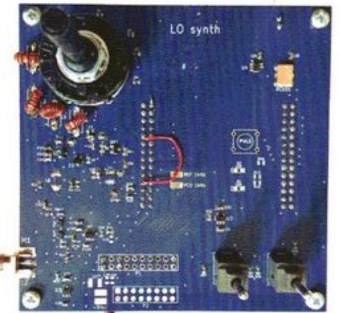
The VCO used for a LO synthesizer
