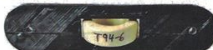
On the left is the 'trap-bone', made by 3D-printer for a T94-6 or T94-2 toroid and related capacitor.
