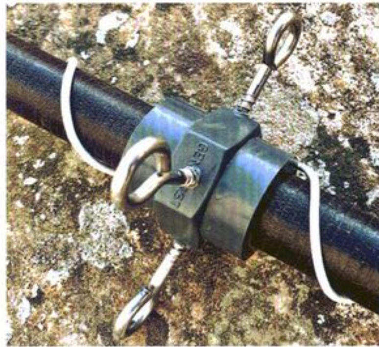
A slightly loose fitted water pipe connector acts as a staying point
