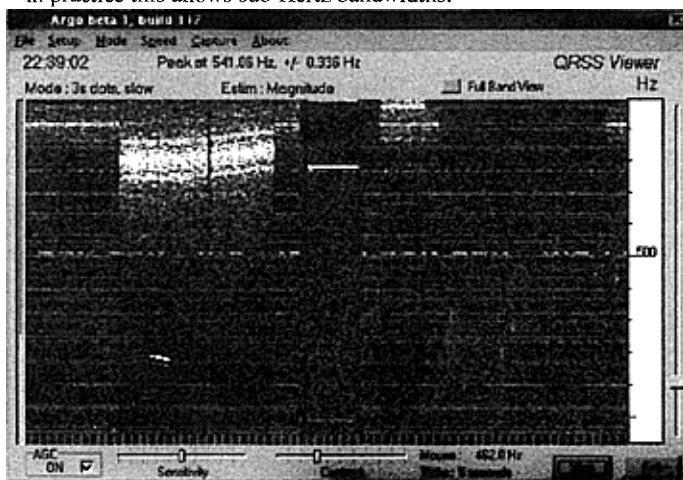
Fig 1. QRSS signal received from 15TGC using the Spectran program. This station only runs 20mW erp. Frequency is displayed on the vertical axis and time on the horizontal axis. The signal on 136.71kHz is showing a slight LF drift of about 5Hz. The other horizontal lines are sidebands from Loran on 100kHz, 36kHz lower in frequency!. The top display is an uncalibrated spectrum analysis of the viewed image.
