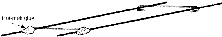
Fig. 2. Spreaders are hooked over the wire, then hot-melted to it.
