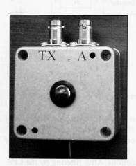
The SWR Bridge on a pcb and built into a small diecast box
