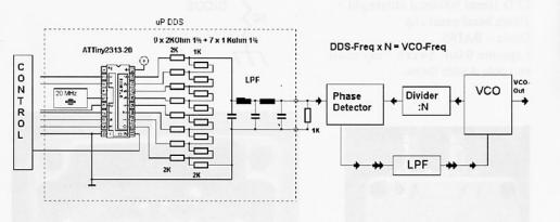
Figure 1: PAOKTS - DDS - Numerical Controlled Oscillator using a Microcontroller
