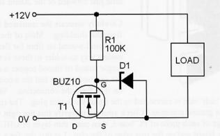
The circuit uses a MOSFET in reverse mode (yes, the drain is connected to the negative of the input!), enhanced by the supply in the correct connection, but remaining in the off-state when the supply is reversed. The MOSFET can be chosen to suit the power demands of the rig. The BUZ10 shown will suit most QRP applications. It has a typical on-resistance of about 60 milliohms so the voltage drop will be less than 100mV up to about 1.5A.
