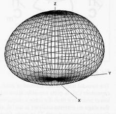
Fig. 3a EZNEC™ FF pattern for aerial of Fig. 1 over perfect ground, no losses (Case A in Fig. 2)
