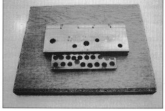
piece of single sided PCB between and gave the punch a good hard bash it produced the desired effect, but it was damaging the back of the single sided board. I thought I would try to punch the islands out in double sided board, so I tried again, this time success, no damage to the islands.
