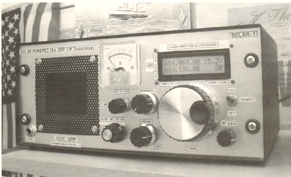
IK0IXI Solar Powered DDS Controlled 20m Transceiver (14 MHz CW transceiver with a QRPProject UniDDS module)
