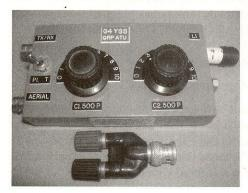
Only then should the top be soldered into place. A 2BA screw through the box wall with its head soldered inside, serves as a grounding stud. The flanges of the two BNC jacks can also be soldered directly to the copper groundplane.
