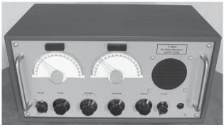
G4DFV has just completed a five valve TRF receiver that tunes LW, MW and two shortwave bands (see picture left). It is based on the receiver circuit of the WW2 'Paraset' with the addition of an untuned RF stage and an audio power stage. Duncan says reproduction of AM commercial broadcast stations is superb and CW and SSB on the amateur bands is ok.
