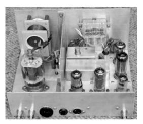
The two brass boxes in the picture contain the 6CW4 crystal oscillator for carrier insertion, and the 6MHz crystal filter. You can just see the two little nuvistors sticking up their cheeky heads. The SSB filter is identical to that used in the Retro receiver.
