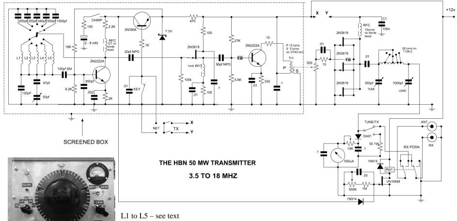
RFC [VFO] – 12t on ferrite bead Tr1 – P 12t. S 5t on bn 37/43 core Pi output coil – 28t T-160-2 RFC [PA] 15t on ferrite bead
