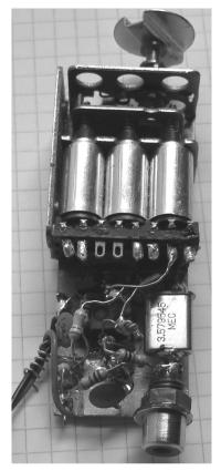
Typical Car Radio Inductance Tuner with approx. DC resistance of windings
