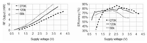
These graphs show the transmitter's power output and efficiency (RF power output as a proportion of overall circuit power consumption) into a 50-ohm resistive load, using different values for the 68k base bias resistor. Oscillation continues all the way down to 0.5V supply! Note that there is no filtering of harmonics and therefore this data is probably over-optimistic, so these graphs should be taken with a pinch of salt (not bleach).
