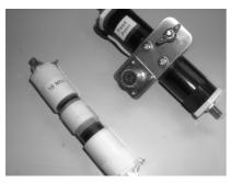
The feed point insulator at base of the antenna is again made from 20mm PVC (in fact I used a piece of 25mm to make it more robust but your 20mm will do ok) Instead of using the bolt through the conduit and aluminium strip to attach the counterpoise wires I fitted and extra screw and nut tightened to it and then a wing nut to attach said counterpoise wires. (See photo) I also used 2 of 4mm set screws and nuts to affix aluminium plate to conduit to stop tendency to swing round.
