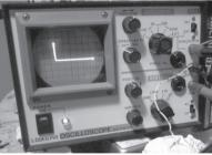
are. Bill writes, "It was so easy to make, just an old heater transformer at 6.3V and three resistors! It allows you to test certain components while they are still in circuit without any power applied. I think it's going to be one of the most used bits of test gear in my shack. The photographs above show the octopus tester in use here, the circular shape trace on the scope shows a 1uf capacitor and the other shows a diode. You can find out lots about it just by 'Googling' octopus tester'.
