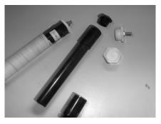
We are using 20mm conduit instead of the American PVC risers to make the loading coils there is a difference of 0.5mm in diameter. (Risers are 19.5mm) The ends are made up of 20mm adaptors and blank plugs both of PVC obtainable from electrical wholesalers. The blank plugs are drilled through their centres to take the set screws and nuts for attaching the rods of the antenna.
