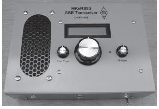
built my MKARS80 in a home-made case so I could include a speaker. The kit comprises a professional quality PTH PCB, all components and case. Knobs are not supplied and you have to drill the case yourself. All this for £50 - incredible value".
