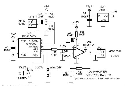
Fig.2 AGC system schematic
