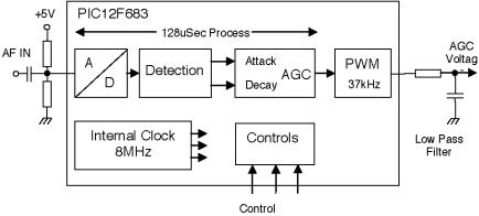
Fig.1 AGC block diagram
