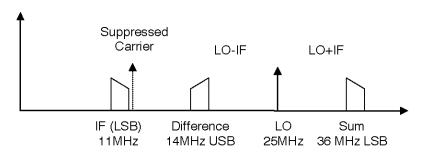
Fig. 1 Frequency diagram for high side LO
