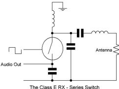
I shared this idea with Wes Hayward W7ZOI and he suggested I try using the MOSFET as a shunt switch - this works as well. The T/R switching and muting is a bit more complex to implement than the series switch version. Experimentation is needed...
