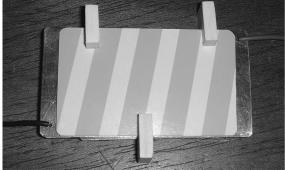
is probably a good idea to cut out the chip in the credit card. The 2 holes at each end should be lined up and a wire soldered to each of the plates. It might be useful to use double sided tape to hold the plates and cards in place during construction. The capacitor could then be wrapped in insulating tape or as I did cut 3 clips out of plastic to hold it together. The capacitor is
