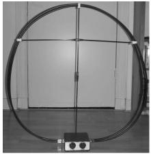
Loop with two capacitor tuner beneath
