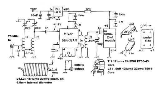
The need to have a listen on 4 Meters CW & SSB necessitated the construction of a simple converter to go in the front of my FT817 rig.
