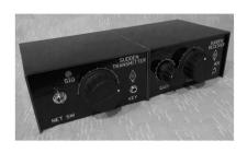
output is 50 Ohms and will need an ATU unless the antenna presents the correct 50 Ohm load. The kit is now available for 40m and we are working on versions for 160m through 20m. The cost is £34 plus postage £2 (UK), £3 (Eu), or £4 (DX), and should be ordered from club sales – see the back page. You can download the full manual
