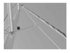
raised by the spinnaker halyard. The wire elements are inside the rope. When the jib was used the antenna was secured to the windward guard rail with no noticeable detuning evident even when the upper parts of the antenna were close to the spars on the mast. Mini pile ups were a treat with best dx being 5N7M and Asiatic Russia worked and ZS and JA that got away without copying our callsign fully!
