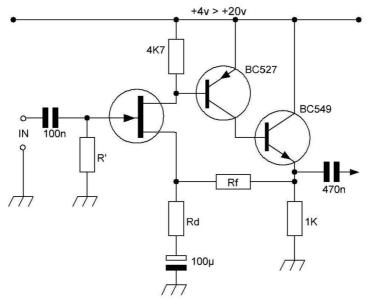
Here's a circuit to lift uV input signals for audio amps to work with. I don't claim originality, its Terry Ritter's design, (www.ciphersbyritter.com) I've used it plenty and it's a cracker. Single rail, 4v and up, a real plus for /M or /P operators.
