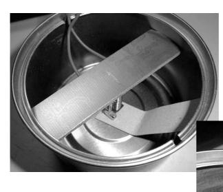
Coil assembly mounting with cardboard spacer
