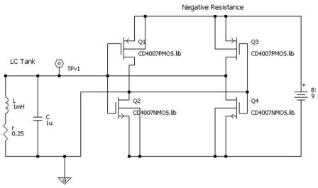
Figure 3. Negative resistance oscillator using the CD4007
