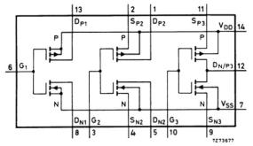
Figure 2. CD4007 dual complementary pair plus inverter.
