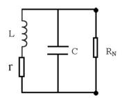
Figure 1. Negative resistance oscillator.
