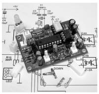
more information and example installations. The X-Lock kit comprises double sided, high quality silk screened PCB, pre-programmed processor, all components, connectors, IC sockets and a comprehensive step by step 14 page instruction manual. Just add 12v and a VFO!
