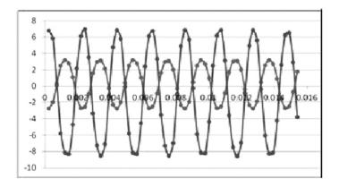
Figure 4. ~500 Hz Oscillator measurements. Larger waveform: Oscillator Voltage (Volts), Smaller waveform: Negative Resistor Current (mA) Time (Seconds)
