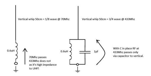
The RF path on either band now takes the lowest impedance path automatically. Since on 433 Mhz a 50cm whip is approx a <sup>3</sup>/<sub>4</sub> wave and has a fairly low impedance in this mode (typically 75 ohms), the antenna has a good SWR and works fine on 433Mhz. On air results are superb!
