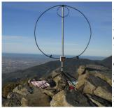
This is the DXLOOP used by **IK5XCT** to make his 5W QSO using his FT-817 with **LU6EF** on 17m in the Winter Sports. The loop is 47½ inches diameter in Cellflex SFC12-50 and covers 40-15m. Stefano says it has 82% efficiency on 17m compared with a full-size dipole half-wavelength high. More pictures and info about it on his website at <a href="http://www.qsl.net/ik5xct">http://www.qsl.net/ik5xct</a>.
