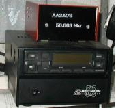
A 6m beacon on 50068lHz PIC16F628 controller, about 1W out to a vertical at 35ft.
