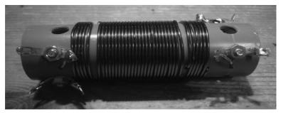
A solid construction is important for a good frequency stability of the RF frontend. Use wires with at least 1mm diameter and keep all connections short. The antenna coil (L1) has 5 turns, the tuning coil (L1 and L2) in total 31 turn with a tap a 6 turn from the end that is connected to ground. You can fix the windings with some glue to improve mechanical stability.
