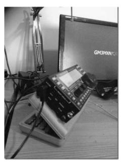
I was unhappy about the KX3 sliding on the bench supported on peg legs, and a noticed that I could purchase from the States a stand which is a bent metal support. Not having heavy gauge metal to make one, and no workshop, I thought about what I could use. I came up with what is shown here; costing nothing. I used an old socket set box. I cut two slots for the peg legs which keeps it from sliding right or left.
