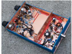
audio amp used manages to get good gain without resorting to the use of a 10uF cap between pins 1 and 8, and the amp has relatively low noise as a result, easily driving a small speaker. Some construction details are at <a href="http://aa7ee.wordpress.com/2013/10/19/the-vk3ye-micro-40-dsb-transceiver/">http://aa7ee.wordpress.com/2013/10/19/the-vk3ye-micro-40-dsb-transceiver/</a>.
