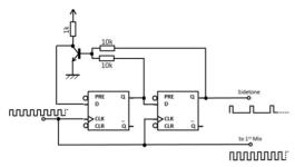
Figure 5 Divide-by-3 for sidetone generation
