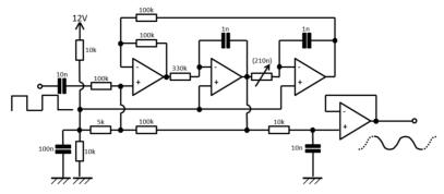
Figure 2 Filter for recovering the fundamental of a 600Hz square wave
