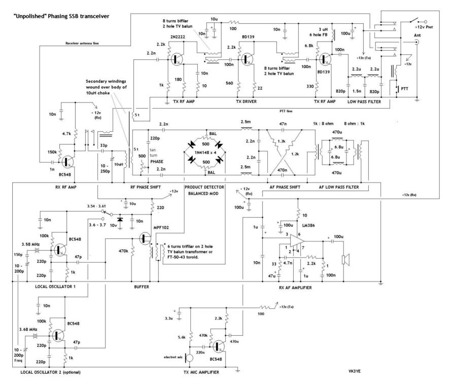
discrete component purist should be able to replace the LM386 with a two transistor audio amplifier for adequate headphone (but not speaker) reception.
