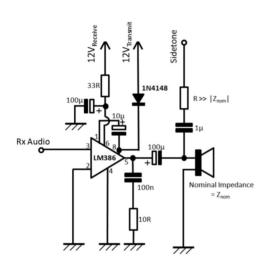
**Figure 1 Injecting Sidetone**
