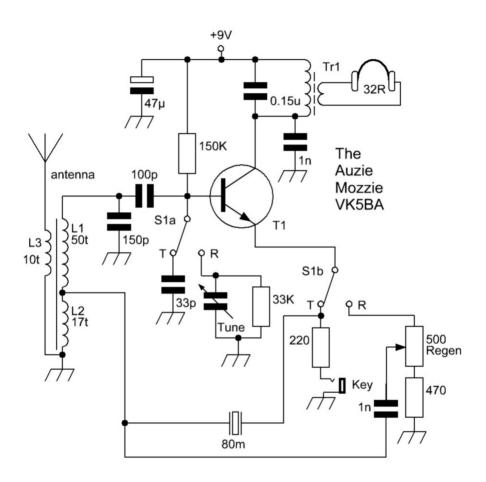
EDITOR'S NOTE: In this novel one transistor transceiver for 80 metres, Malcolm uses some local Australian parts. It is offered as a circuit suggestion leaving readers to experiment and find local equivalent parts for themselves.
