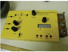
designed and the hard to fit SMD devices are already pre-soldered onto the board so I was pretty confident that they were all ok. Quite a lot of dry joints later and an SA612 replaced, brought the RX to life, The TX - once again a few dry joints and bad soldering made this part function. So now having a working PFR3 how could I break it!!!.
