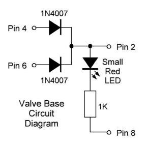
The results were interesting; with the 5Y3 and without a load on the psu, 330V ht was obtained. With the diode substitute, 355V was reached again with no load. I have not had the opportunity yet to do tests under load conditions.
