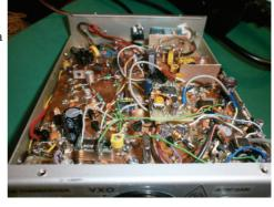
The audio filter is a OK1CDJ 2012 project. I found it as kit, sold on Ebay and made using SMD components. I built it with normal size components. It works fine and finally I have good reception "stand alone", without help by Datong FL-3 audio filter. The transmitting chain is very simple and it gets more than 1 Watt out. A semi-break in circuit allows "hands free" operation. I made more than 40 2XQRP QSO in few days, including G3VTT, GM3JKS, UR5TKM, SM7RYR/7."
