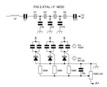
replace C8, C9, & C10. Feed each MV109 through a 100k resistor and then feed all three 100k resistors from a 100k pot from the new 5.1 v zenered supply with a 0.01uf across the pot output. As per the circuit diagram (fig 2) and photo right.
