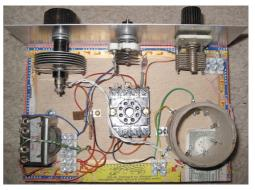
even maybe a bit of SSB! Fine stuff for a first radio for my friend I thought. (Actually, I am such a liar; I spent ages getting it to work satisfactorily... The output transformer and the bypass capacitor went through a number of revisions before I was satisfied and I fiddled with the HT too before settling on 27V - 3xPP3s).
