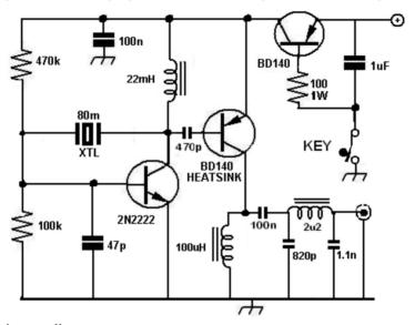
The base is a small tobacco tin. It may be practical to make the transmitter work on another band by changing the crystal and PI filter plugin board? The output power can be adjusted by altering the supply voltage. If you run it on 19v at 5W as I do sometimes using a 2W 100 ohm resistor in series with the key would be better as my quarter watt one gets too hot. Also note the BD140 needs a good heat-sink.
