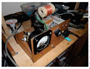
Just a note to say how much I enjoyed the Valve QRP day over Easter. I was looking for an excuse to use my 6V6 co/pa TX once again with club crystals 7025 and 3560. It was from a 1960's PW design. RX used was an IC703 and aerial W3DZZ. Manual aerial changeover was deployed. I first built the
