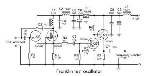
Its construction is not critical but wiring and rigidity should be considered and leads kept as short as possible, dead bug, PCB construction is up to you, a metal box should obviously be used with suitable connections for the coil or tuned circuit under test.
