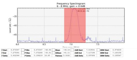
Now as I wrote previously, I am not claiming that we have a spectrum analyser with tracking generator here and the accuracy of the dB markings may not be massively accurate. However, if you wanted to build a filter from one of the many published designs, and needed to check that it was actually working where it was supposed to, you would get a pretty good indication plus some idea of the bandwidth. Much better at least than you would if you had no test equipment.
