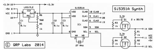
QRP Labs also produce an Arduino Shield for the Si5351A Synth kit, with an onboard QRPp PA and sockets for a plug-in LPF. Example sketches demonstrate how to configure the Si5351A registers for a desired output frequency. These examples will be useful for anyone wishing to write their own code to control the Si5351A, see <a href="http://qrp-labs.com/synth/si5351ademo.html">http://qrp-labs.com/synth/si5351ademo.html</a>
