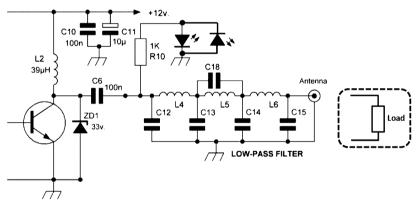
Figure 4 Revised LED RF Indication for the Sudden Tx
