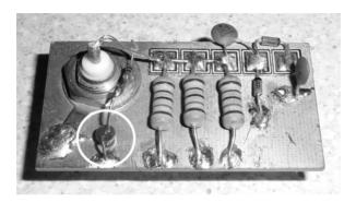
One of my dummy loads including the LED RF indicator is seen, from the component side, in Figure 1. The LED is highlighted by the white circle. The system is otherwise as described in the Sudden Tx construction notes, [2], including the voltage-doubling peak detector circuit.
