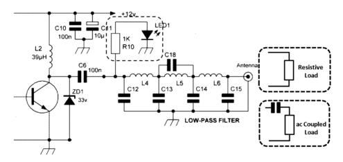
Figure 2 Elements of the Sudden 2 Tx Output Stage and its Load
