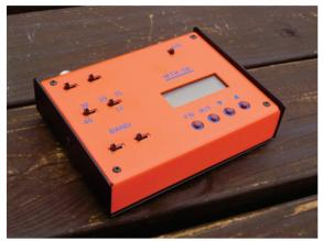
KD1JV's kit for 2015 was the fourth in the MTR series, called the MTR-5B. The rig now includes operation on five bands, a backlit four line LCD and optional rotary encoder.
