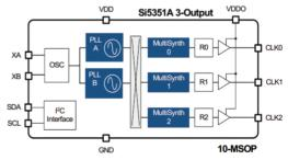
range 600-900MHz. That frequency is divided down by a "MutliSynth" divider. Each of the three outputs has its own Multisynth divider, and there are two PLLs. The outputs also have a further divider stage (labelled R0, R1, R2 in the diagram) that divides by a power-of-2 between 1 and 128. The PLL multiplication and the MultiSynth division are both fractional, which allows very high accuracy of the output frequencies. However the
