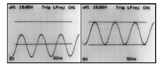
Figures 3 Output Voltages with a.c. coupled (left) and resistive (right) loads
