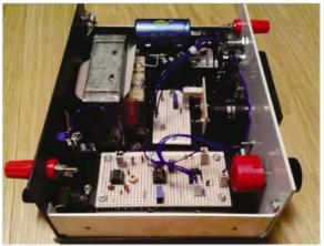
varistors and for 're-forming' antique electrolytic capacitors. It supplied HT to my home brew valve RX without any problems.
