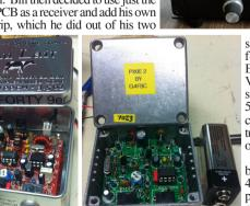
stage VFO fed into a BC108 and VN10 PA stage to give 500mW all
