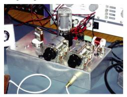
Those declaring the use of valve transmitters were G3XIZ, G4GIR, G4AQS, G0ILN and G3VTT. On 80m I employed a CO/PA using a couple of 6V6s producing 5W and on 40m a single 6V6 running 2W both feeding a G5RV aerial at 15ft. The receiver was a Drake 2-C. See photo. Many thanks again to the organiser for another enjoyable weekend! 72/73 Derek **G3NKS**
