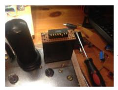
Train it with a kink to fold back in neatly into the case later when the lid is screwed on. Insulate the crystal cases with tape if the metal plates are still inside your case otherwise they will short the pins two connection pins. Tin these wires and solder to the line of joined crystal legs and the 1mm copper wire. Carefully ease the whole assembly inside the crystal case and screw on the lid.
