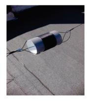
The balun construction next the loading coils for the dipole.
