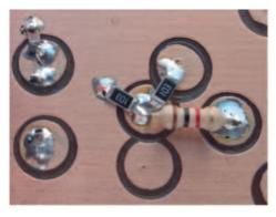
The picture hopefully demonstrates the technique and, in case you are interested, shows a partially completed circuit for G3UUR method of crystal motional parameter measurement (QEX Jun 1995 p20).
