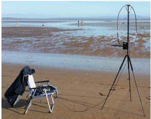
very quick to put up and pack away, takes up little room when stowed and for portable operation is clearly an effective alternative to wire antennas". Ron plans to build a slightly larger version to extend low-end coverage to 40m and believes that with remote capacitor tuning, it would be an ideal solution for those with limited space for conventional antenna systems.
