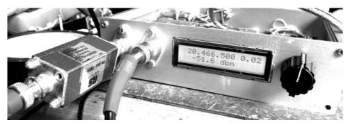
This is a 10MHz low pass filter, so the attenuation is shown as high – just as you would expect at 20 MHz.
