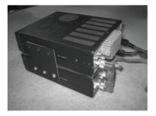
The mounting holes in the  $3/32 \ge 342 \ge 4$ -inch aluminium plates were laid out to match the mounting holes on both the transceiver and tuner with the TS-50 sitting unsupported atop the tuner. The plates were secured with the metric bolts that came with the radio and mounting bracket.
