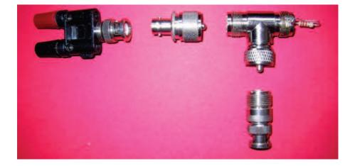
A little research told me that resistors between 1K and 10K would make a suitable drain resistor without affecting receive or transmit modes. I thought that I could install the resistor outboard of the radio and not have to find room in the innards.
