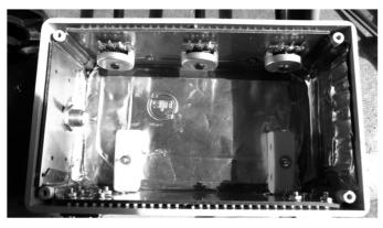
In the corners you might be able to see adhesive copper gardening "slug tape" to complete the screening. This is thick enough to solder to and is probably more effective used in the shack than when protecting my strawberries.
