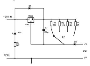
My aim was to have current output ranged in a binary sequence of 25 mA, 50 mA, 100mA and 200 mA with current set by a four-way rotary switch.
