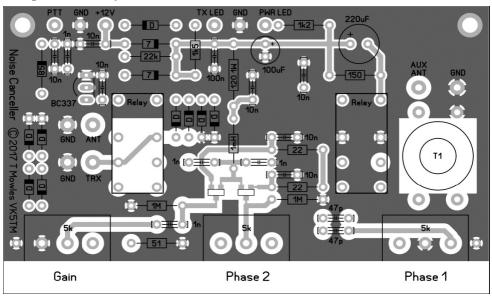
The diodes marked "D" are 1N4148's, "7" - 1N4007's and "85" - BAT85. (1N4007's were used as that is a standard component in my workshop, 1N4001's, 1N4002's etc should be equally suitable and a 1N5819 was used for the BAT85). The pcb is available from the author (see website) for \$10 AUD (Australian residents need to add GST) plus Post and Packing and a kit of parts, excluding case, connectors and knobs, should be available by the time you receive this edition of Sprat.
