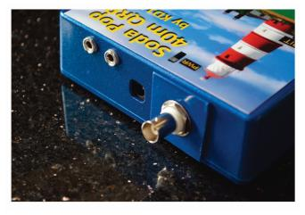
lacquered that too. The whole thing was assembled after the front panel was stuck on with red Spraymount.
