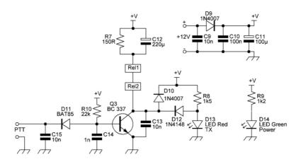
Fig 2 - Power supply and PTT section
