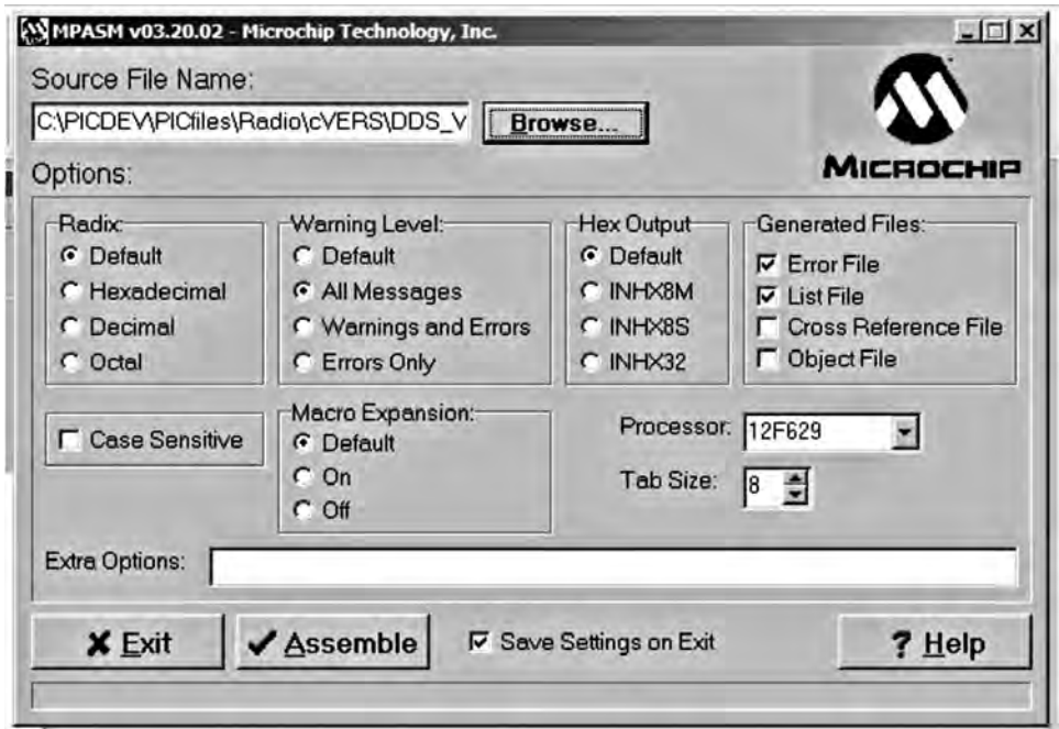
MPASM screen showing selected .LST file and chip type.
