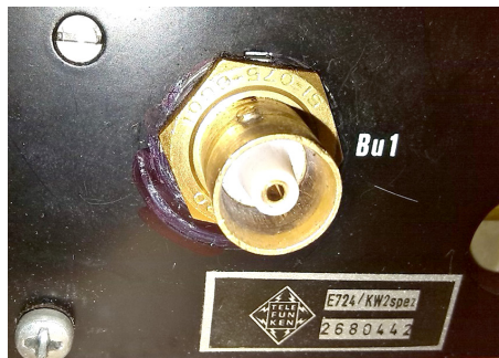
The C connector socket on the EK 724 that has to cope with a home-brew plug
