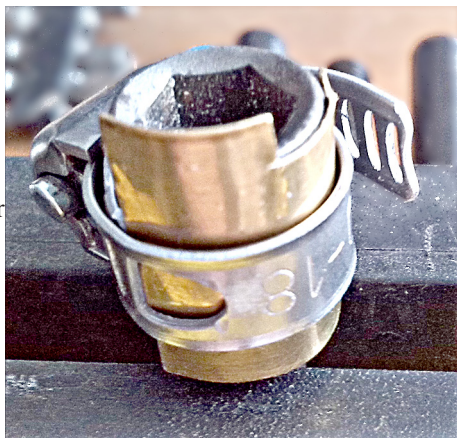
Bending the brass sheet into shape around a smaller cylinder with the help of a Jubilee clip
