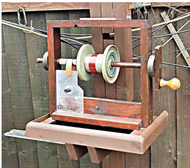
The winding mechanism, note the 'slip-ring' arrangement to connect the signal into the wire
