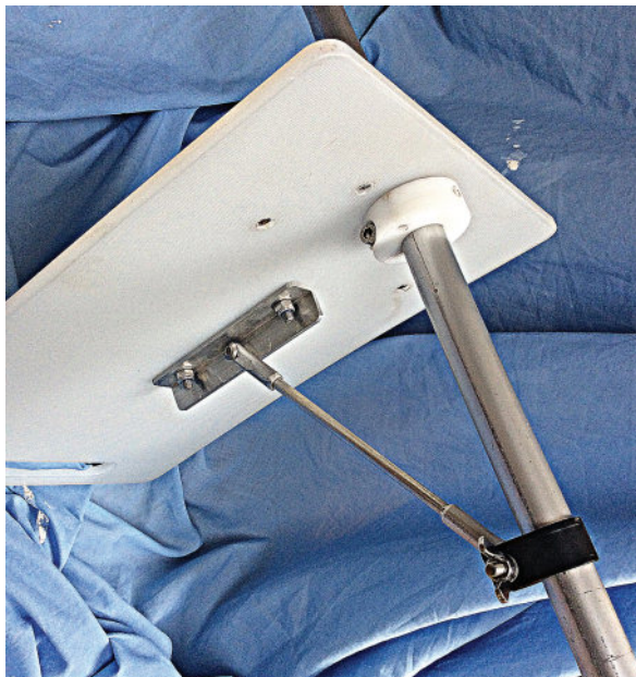
The ‘desk’ is braced with a clamped aluminium rod
