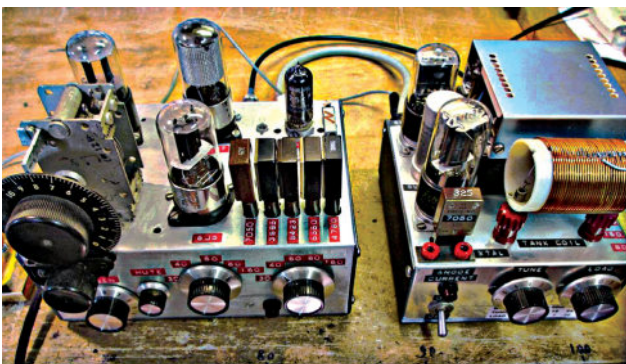
The setup used by Wim PAØWDW – Regenerodyne Rx and a 6V6 CO/PA Tx
