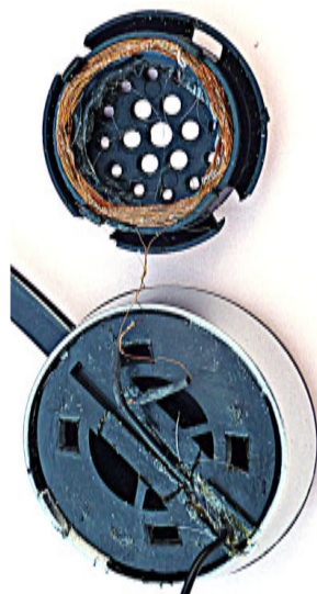
Figure 1: Remove the original 'loudspeakers' as in Peter's article and replace them with the biggest coil you can fit in the empty space.
