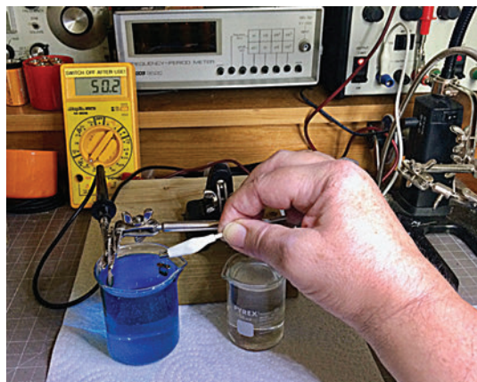
Fig 4: Plating progress, it doesn't need long
