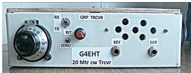
The original 20m transceiver design was a complete VFO driven unit shown here. But lack of time precludes a design explanation this time.
