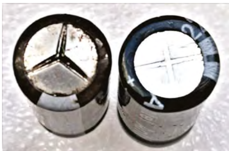
A 'blown' electrolytic capacitor. The one on the left has ruptured the weakened can end, which prevents it exploding completely.
