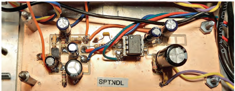
The amplifier board installed in a radio which I call the Spilsbury Tindall Replica
