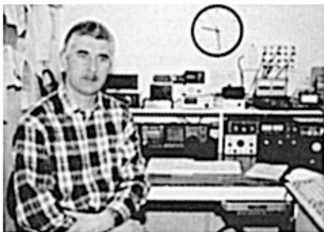
Robin, G4GIY, in his shack, behind him (top shelf) is a DTR3 (behind his shoulder), sundry SWR meters and RF analyser etc, FT290 and TNC for packet and a balanced ATU. On the bottom shelf is an IC-756, OHR Spirit and MFJ tuner on top, FC-902 ATU and a converted CB rig for 10m FM.
